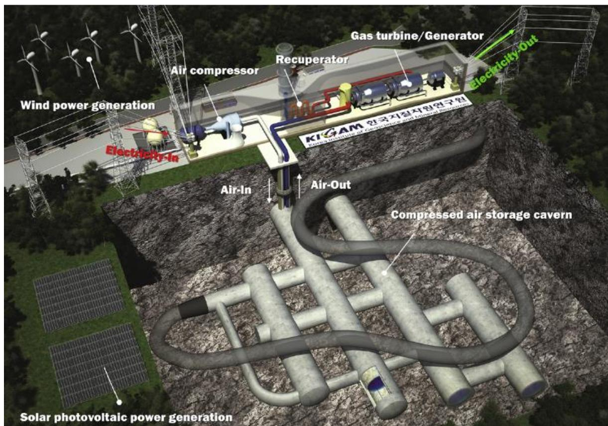
Figure 1 Overview of a possible layout for a CAES-facility with underground caverns. (Kim, et al., 2012)
