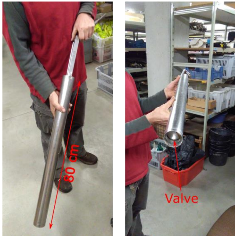
Figure 10 Pictures showing the riverbed auger with indication of the length and the closing valve.
