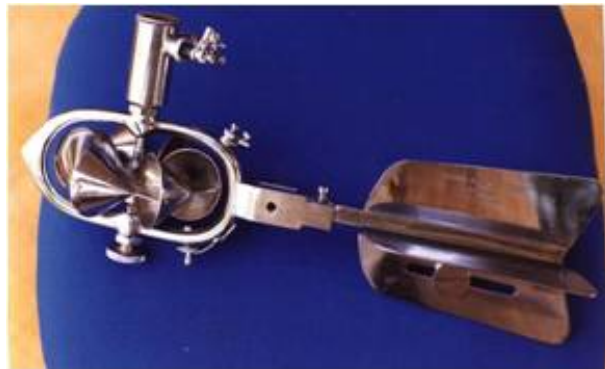
Figuur 12 Cup-type rotor Bron: Cwprs [19]
