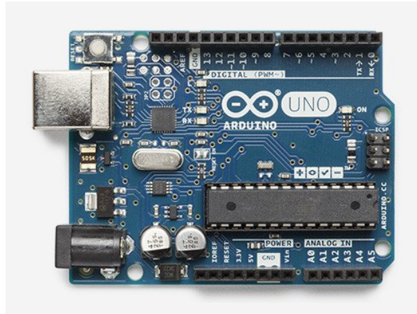
Figuur 17 Arduino Uno board Bron: Arduino [9]
