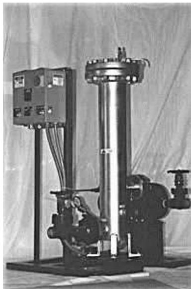
*Figure 14 Liquid Process Systems, Inc. (LPSi) hot oil filtration unit,
