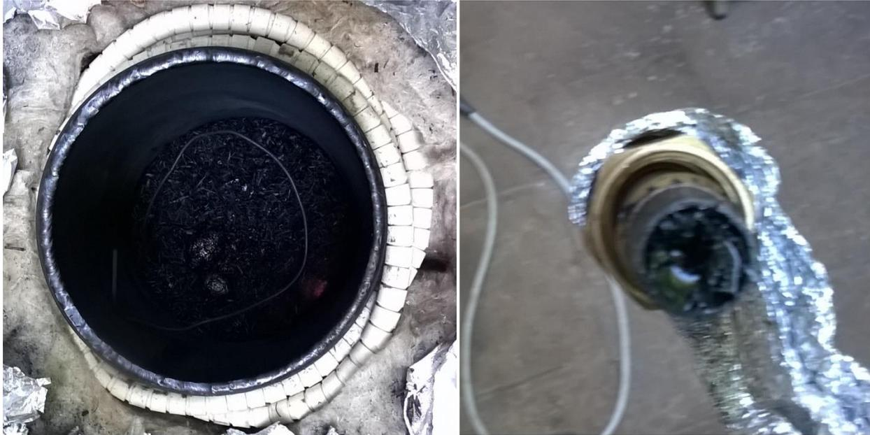
*Figure 4 Char collection in the reactor chamber (left) and exhaust tube clogging (right)*
