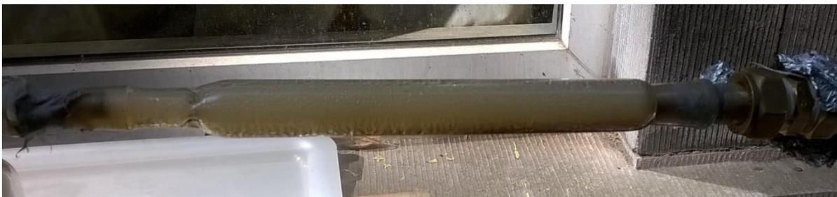
*Figure 3 Collection of droplets in the connection tube*
