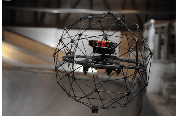
Figuur 13 Elios cage protected drone (Flyability)
