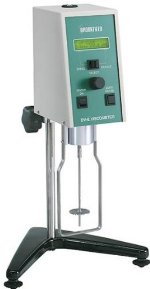
Figuur 42: Brookfield DV-E viscometer. [39]
