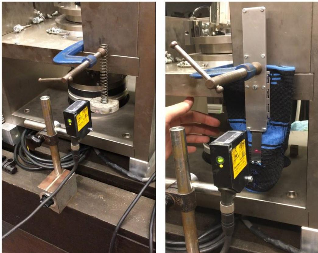
Figure 6.8: The test without the orthosis (left) and with the orthosis (right).
