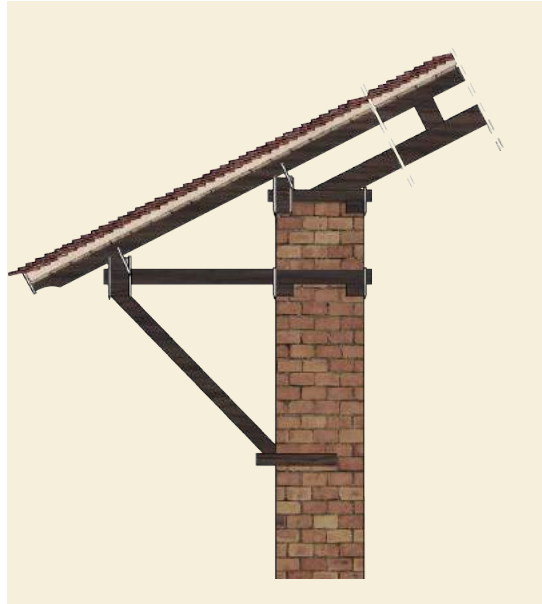
interlocking roof structure
