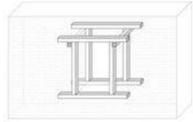
Scale 1/50 Surrounding bricks adapted to double framed window.
