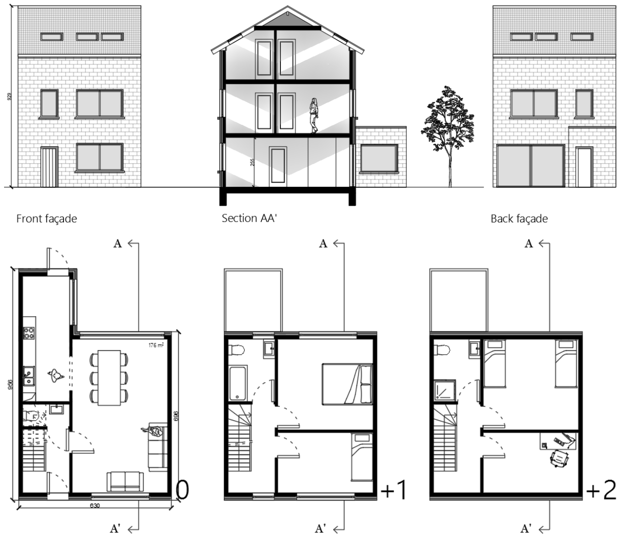
Figure 36: Floor plans, façades and section of the conventional house in original stage
