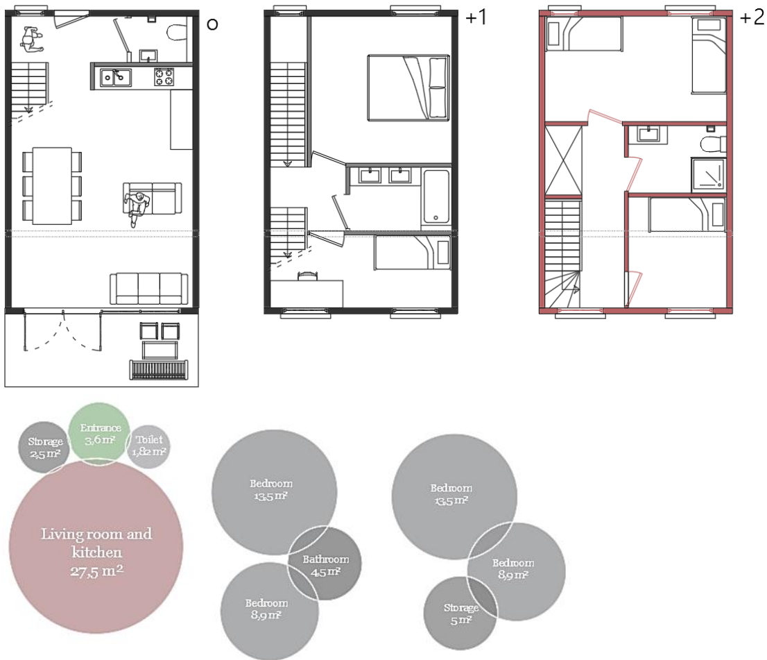
Figure 49: Floor plans and corresponding floor areas of the expandable house in the 'Children (2)' scenario
