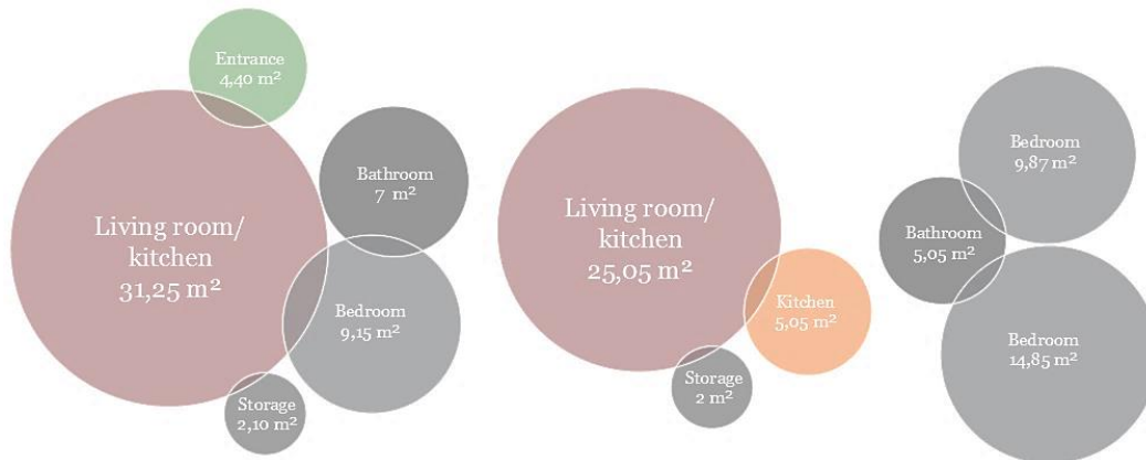
Figure 41: Different functions and corresponding floor areas of the 'Kangaroo dwelling' conventional house
