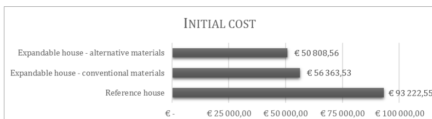
Graph 5: Comparison of the initial cost of expandable houses (cores) made of alternative and conventional building element and initial cost of the conventional reference house
