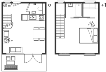
Figure 69: Floor plans of a conventional house and of the core house of the expandable house
