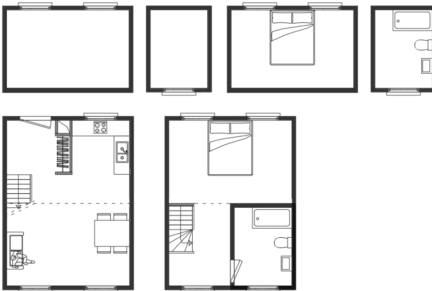
Figure 51: Floor plans of four base modular volumes and a core house resulting from a combination of such modules
