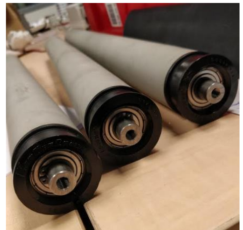
Figuur 28: Conveyor rollen van TVH conveyor (Dalgan, Defoort, Lambrecht, & Mattelaere, 2018)
