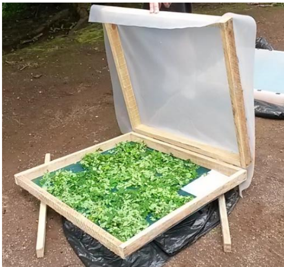
Figure 6: A hand-made solar dryer for leaves, suitable as a low-cost option for rural communities and households. The frame is made from plywood, black bags create a heat absorbing base below and a UV-filtering plastic is placed top the dryer. The dryer is not in direct contact with the soil, but remains suspended above it (credit: B. Peddi).
