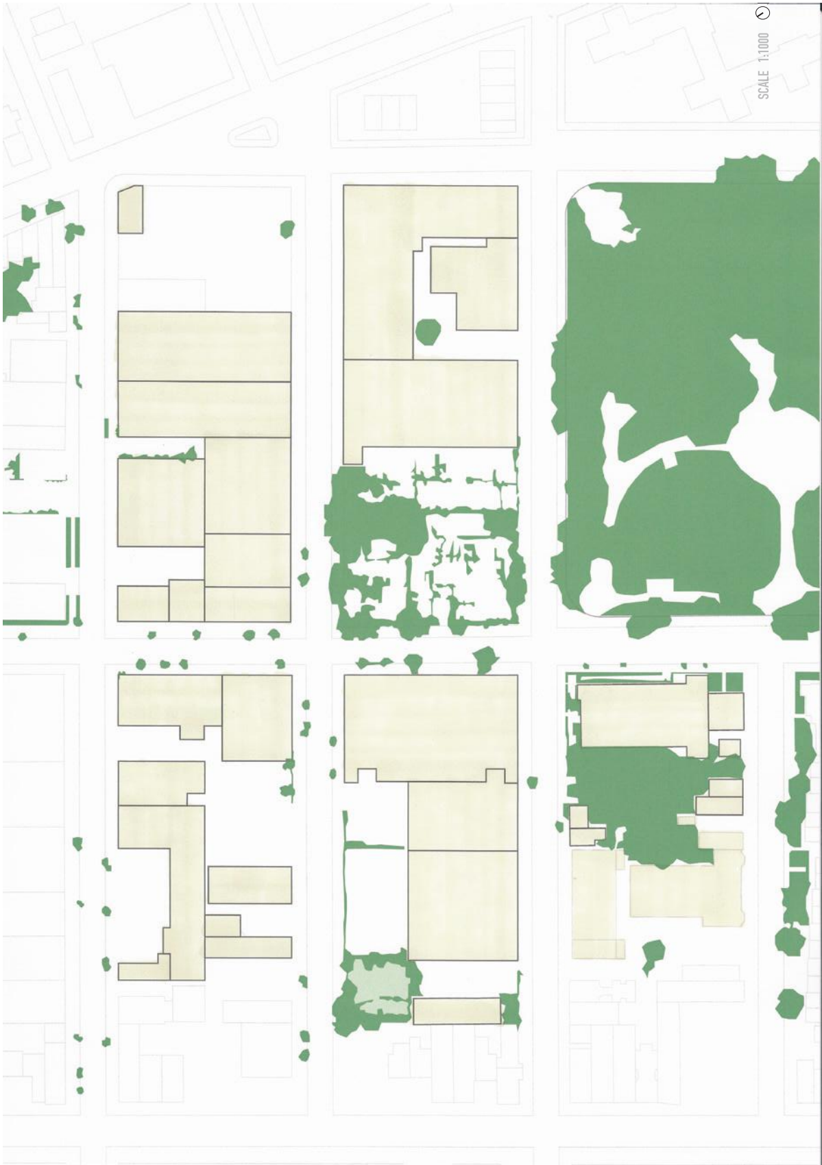
FIG. 67 : NATURAL PERMEABILITY AT SITE 1 (R-SITE, RICHARDS STREET NORTH) : VEGETATION, TREE CANOPIES, BIOSWALES & OVERGROWN ROAD CRACKS
