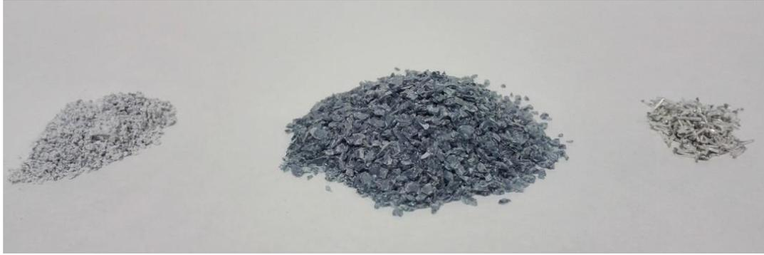
Figure 42: Different fractions obtained after disc milling, sieving and magnetic separation. Left: fine plastic flakes. Middle: coarse plastic. Right: electrodes.
