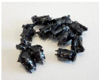
**Figure 39: LEDs after thermal treatment at 500 °C in argon atmosphere.**
