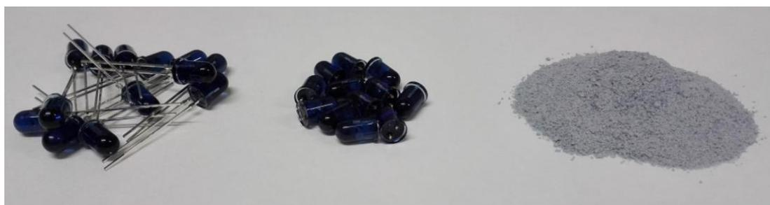
**Figure 37: Left: original LEDs; Middle: LEDs with cut off electrodes, Right: grinded (mechanical mortar grinder) LEDs.**
