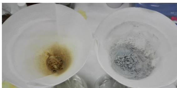
**Figure 41: Metallic (left) and plastic (right) fractions after mortar grinding, density separation, filtration and washing.**
