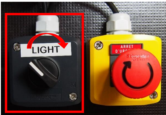
Figure 52 Light switch Source: own work
