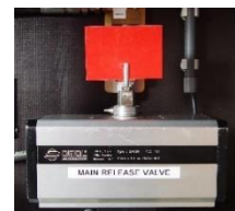
Figure 89 Main release valve, open position Source: own work
