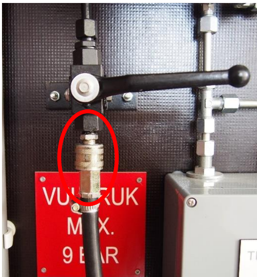
Figure 58 Compressor connected on pilot cylinder filling piece Source: own work
