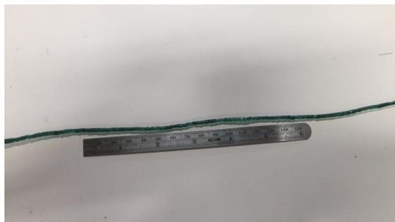
**Figure 5.2:** Filament produced from JT5000 with stoichiometric ratio  $r = 0.5$ .
