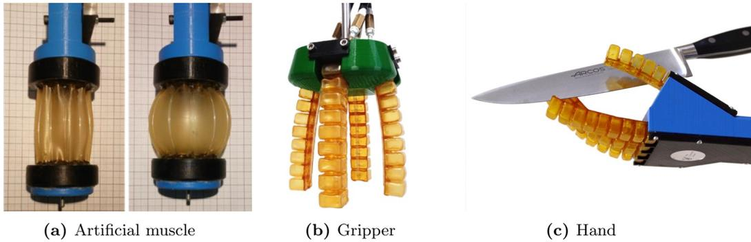
**Figure 1.2:** Different SH pneumatic actuators developed at VUB. The inflatable cells are clearly visible in the hand and gripper [1][2].
