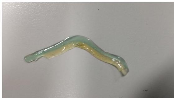
**Figure 5.3:** A small piece of a multi-material print is successfully obtained. JT5000 (yellow) and JT3000 (blue/green) are printed next to each other.
