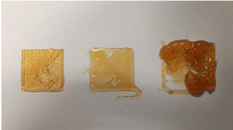
**Figure 4.7:** A test specimen of 20 mm×20 mm printed at different extruder temperatures: 117 °C (left), 120 °C (centre), 125 °C (right). A better print quality is achieved at low temperatures. Note that the number of layers printed is not equal in the different samples, due to the filament buckling. The print at 125 °C is above the allowed temperature, but is added for comparison purposes.
