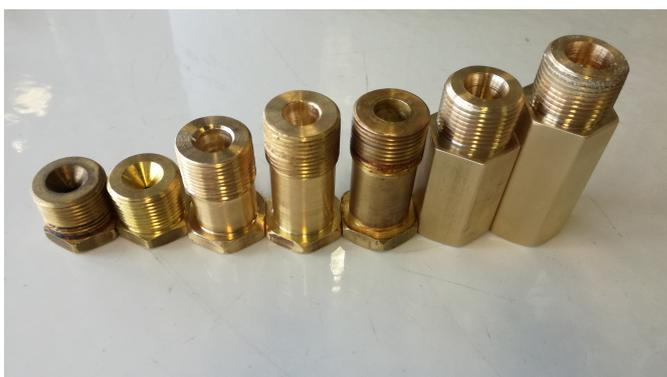
**Figure 3.4:** Evolution in the die design from left to right. The newer dies have an increased land length and smaller angle of entrance.
