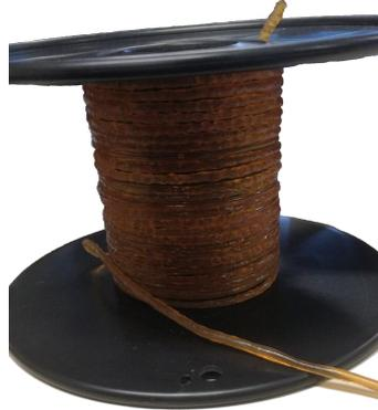
**Figure 3.9:** A batch of filament produced during the filament optimization process. Shark-skin is still present but the general diameter variations in the bulk of the material are good.
