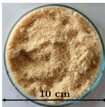
**Figure 3.5:** The DA material is brought to below its  $T_g$  by using liquid nitrogen and then grinded to produce fine particles.
