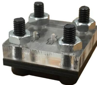
*Figure 34: Prototype of the final holder. The holder features guiding holes for the drill bit and threading tap to precisely align with the cut holes.*
