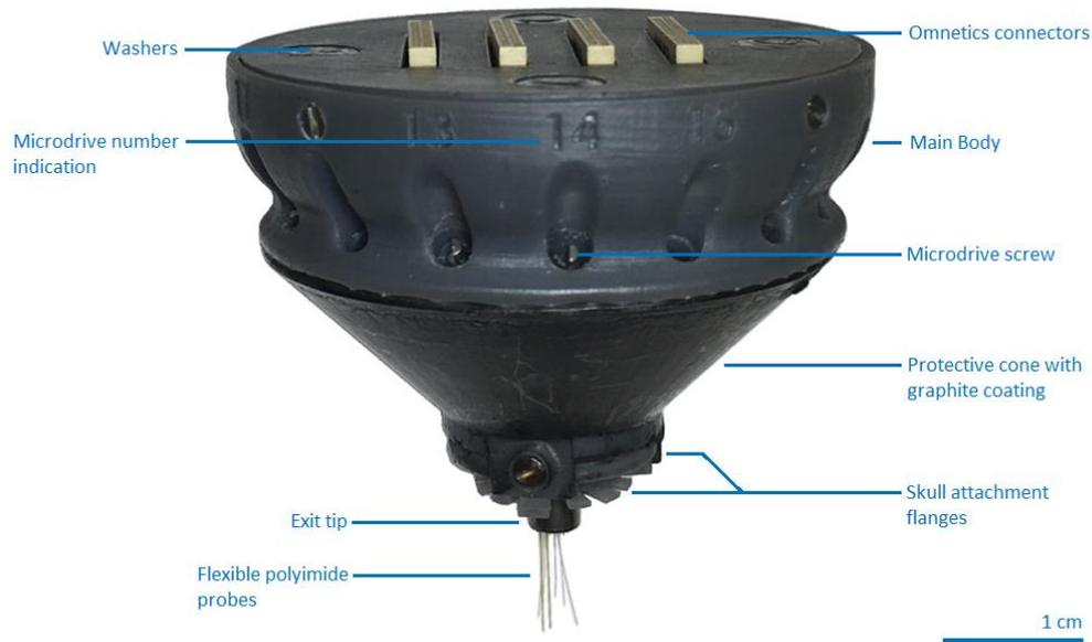
*Figure 35: Final version of the hyperdrive. It contains 16 microdrives indicated by numbers. The probes are lowered through the exit tip by turning the microdrive screws. The graphite coating creates a Faraday cage around the electric components. The Omnetics connectors send the recorded signals to the outside. The skull attachment flanges are used to connect the device to the rodent's skull. The removable cap with magnets is not shown.*
