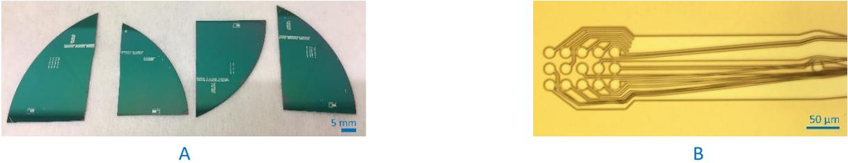
Figure 9: Possible problems that can occur with lift-off. A) All metal paths are lifted-off from the substrate. B) The resist was too long developed and loosened from the substrate. In this case the metal tracks would fuse together when depositing.
