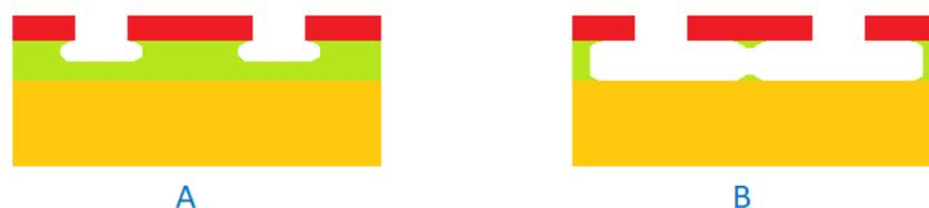
*Figure 8: Illustration of resist development problems. The lift-off resist is shown in green. A) The lift-off resist is not developed long enough causing a lift-off of all deposited metals. B) Too long developing causes drift of the top resist layer or a fusion of the metal tracks later on.*
