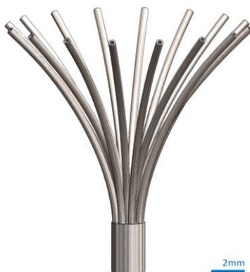
Figure 36: Proposed exit tip design for easier insertion of polyimide tubes.
