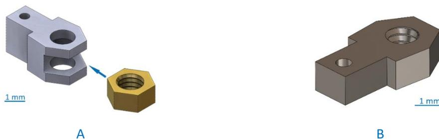
Figure 27: Custom designed shuttles. A) 3D-printed shuttle with nut holder (grey), M1.2 nut (yellow). The arrow indicates the assembly of the nut and its holder. B) Stainless steel shuttle, the height is halved compared to the assembled version, increasing the travel length by 1 mm.
