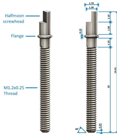
Figure 26: Custom made microdrive screw adapted from Kloosterman et al. [8]. 3D-view of the hyperdrive screw and side view.
