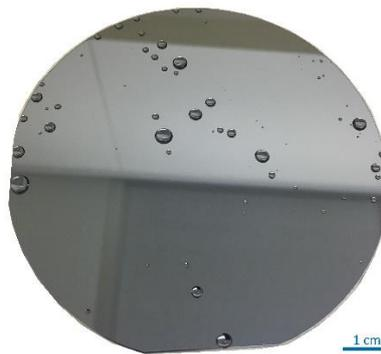
*Figure 14: Silicon wafer with water droplets. A hydrophobic reaction to the substrate surface appeared, which indicates that the native oxide layer was sufficiently removed by buffered hydrofluoric (HF) acid.*
