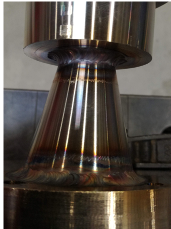
Figure 5.13: Connection welds between back-plate, conical duct and left hub
