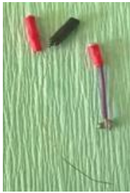
Fig I: illustration of a bipolar depth electrode (left) and scalp electrode(right). The bipolar depth electrode is used for measuring EEG-signals inside the seizure-focus, whilst scalp-electrodes are employed to cancel out artefacts and correct for non-epileptic brain-activity.
