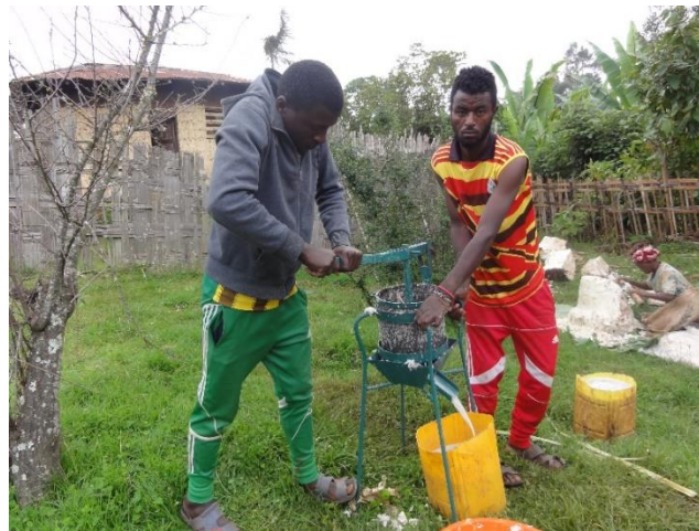
Figure 5.1 Squeezing equipment from Wolaita Technology Transfer center to obtain bulla (own photograph)
