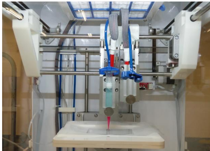
Figure 3.3-3 Cartridge and nozzle mounted onto printhead
