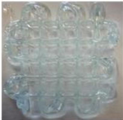
Figure 6.5-7 3D structure, Cellink start, 25G conical nozzle, 60 kPa, 15 mm/s feed rate, 40% infill, 0.15 mm layer height. Dimensions (2 x 2 x 0.5) cm
