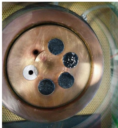
Figure 4.1-1 Prepared HA samples for SEM
