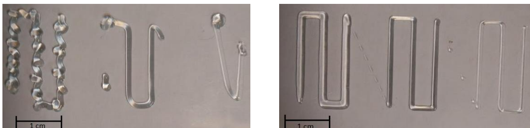
Figure 6.2-1 Left visual calibration, right with a piece of paper. Printed with Cellink start at 60 kPa, 0.25 G conical nozzle and respectively 2, 5 and 10 mm/s
