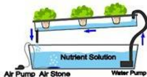
Figure 6: Simplified representation of hydroponics technology in the BySpire facility, the Nutrient Film Technique: at the top a plant production system with irrigation pipes is shown, the drained water is collected in the bottom reservoir, and is recirculated to the plant production system which the necessary nutrients and oxygen (NoSoilSolutions, 2018).
