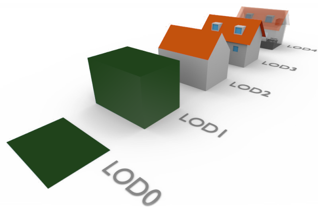
Figure 4. Representation of a dwelling in different Levels of Detail (LOD). (Vlaamse overheid, 2018)
