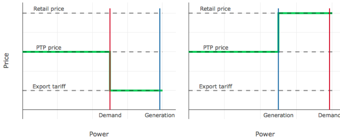
Figure 4.1: Left: consumption and export prices when microgrid PV generation exceeds consumption. Right: consumption and export prices when microgrid consumption exceeds generation.
