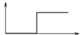
Figure 3.1: Shape of the perceptron activation function, shifted from the origin by the bias term b .
