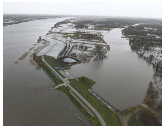
Fig. 2.5. The Kruibeke polders, Flanders' the largest controlled flooding area (Sigma Plan, 2018)
