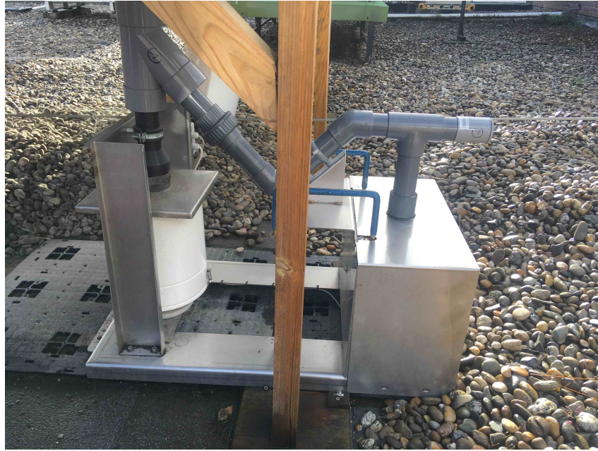
Figure 3.3: Each tray has a double pluviometer at its outflow (picture by Ewout Vereecke).
