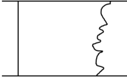
**Figure 2-10 Cylindrical pore on the left and tortuous pore on the right**
