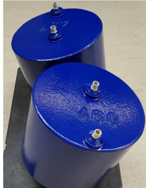
**Figure 2-2 Left: Schematic representation of an AGMD module, Right: Two AGMD modules from Aqualstill**
