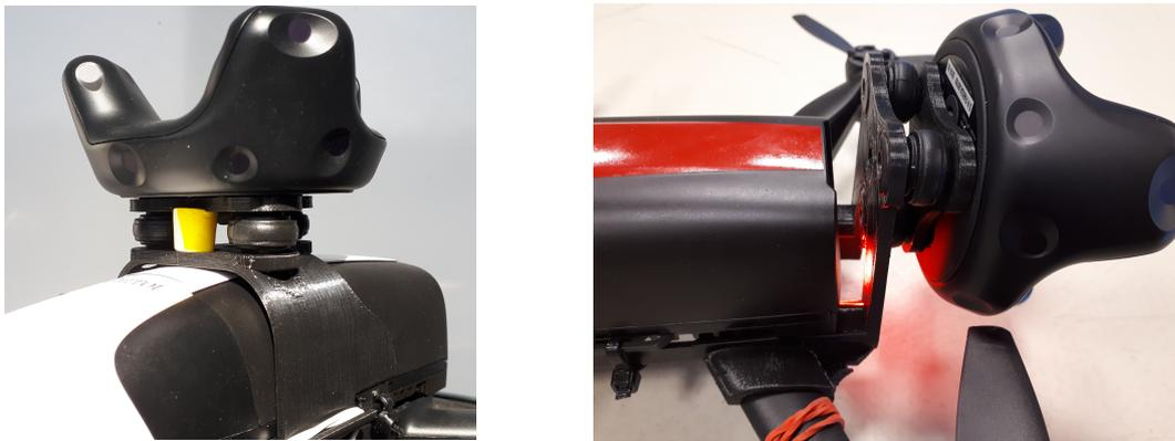
Figure 2.2: Two alternatives to tracker mounting: on top or at the rear.
