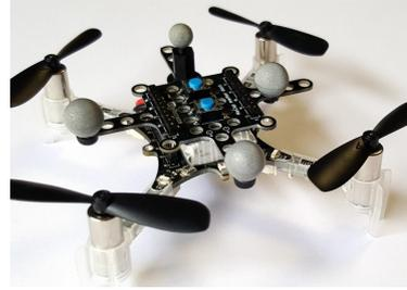
Figure 1.2: Reflective markers used for localization in the Vicon system depicted by the grey balls [10].
