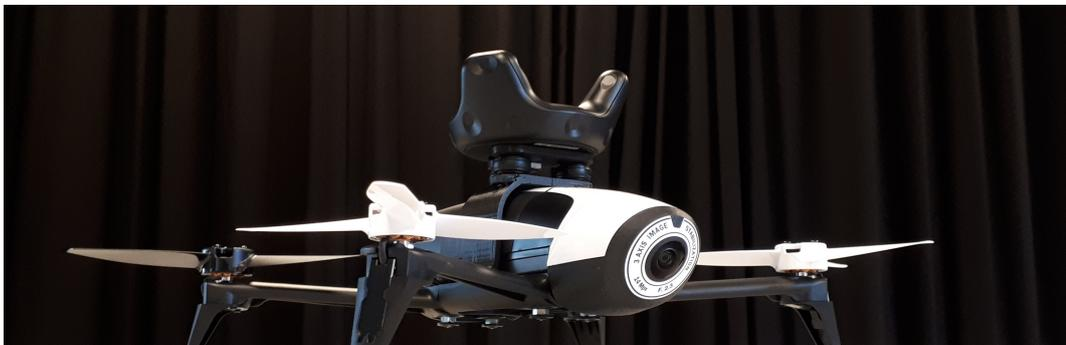
Figure 2.1: The selected drone with tracker from the Vive localization system mounted on top.
