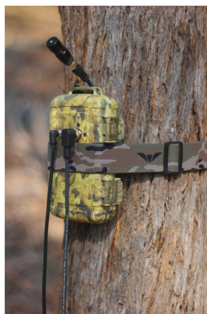
Figure 4.2 Example of a full spectrum passive bat detector. (Anabat Swift bat detector, Titley Scientific.)
