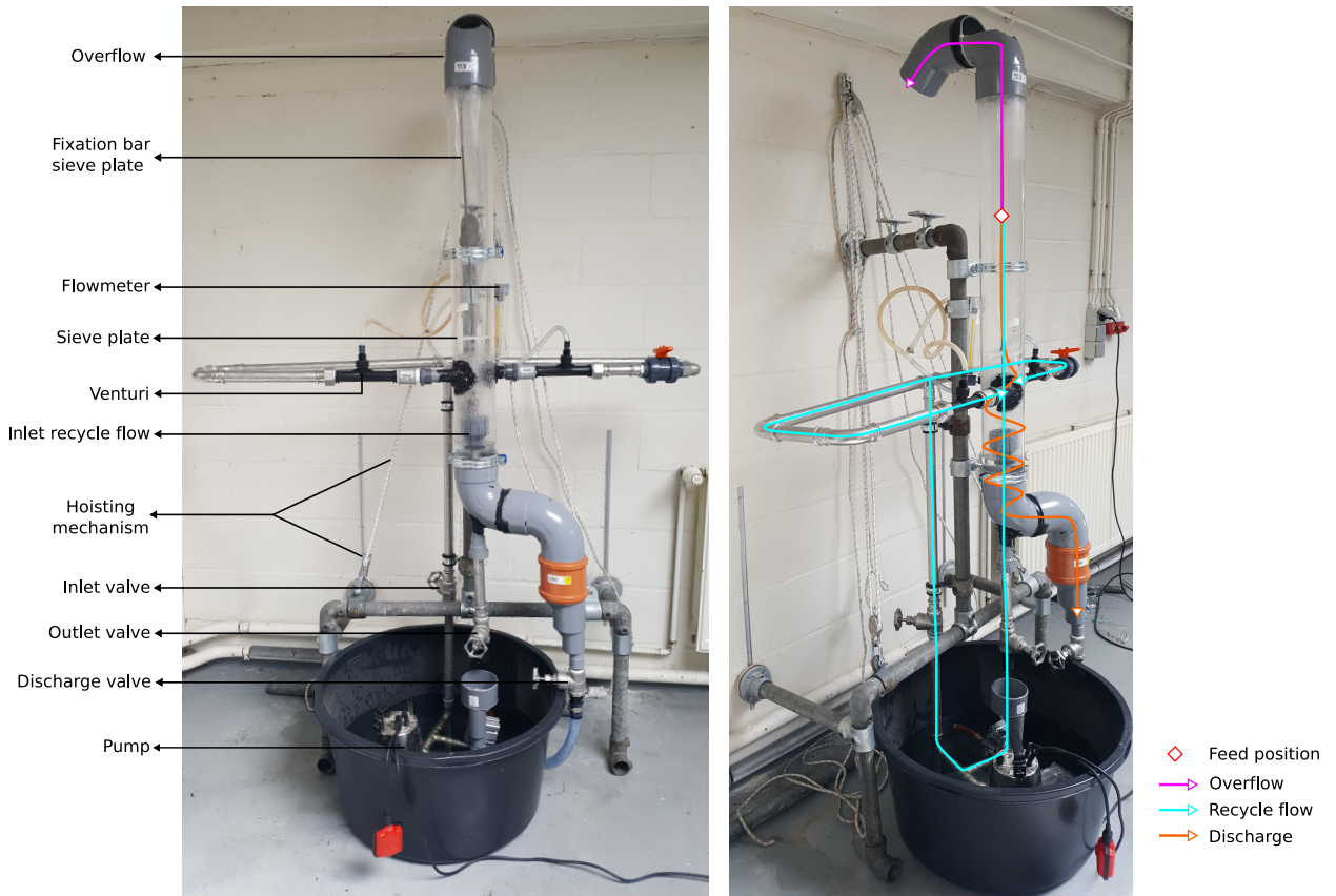
Figure 4.15: Images of the constructed flotation installation with clarifying information about the different components (left), and illustration of the different flows (right).
