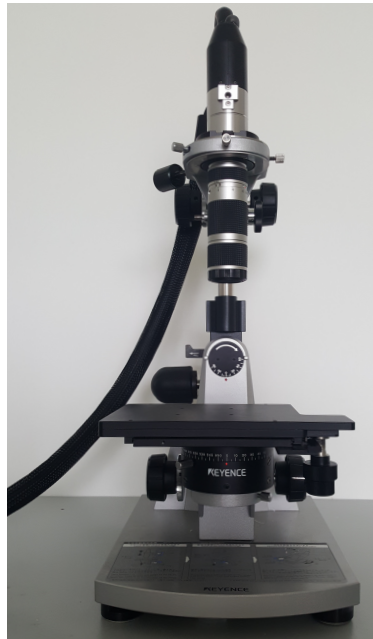
Figure 4.8: Image of the Keyence VHX-500FE Digital Microscope used for the shape characterization of the microplastic particles considered during this research.
