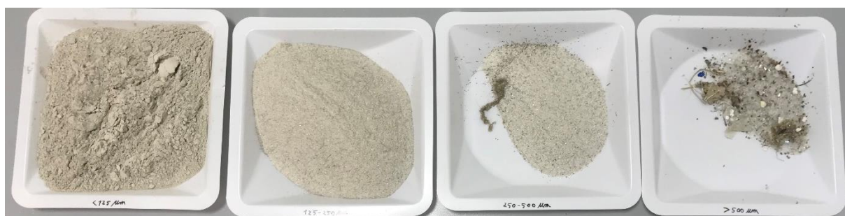
Figure 10: Picture of the four fractions after sieving the phosphor waste, from left to right: < 125 \mu\text{m} , 125 - 50 \mu\text{m} , 250 - 500 \mu\text{m} and > 500 \mu\text{m} .
