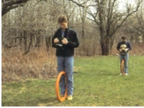
Figure 2.6: Typical measurement set-up with the EM34-3. Figure retrieved from [Geonics, 2012].
