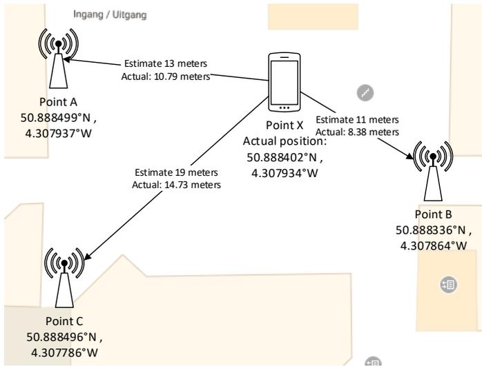
Figure 34 - Trilateration positioning in larger open spaces such as entrance halls (Pediatrics UZ Brussel)
