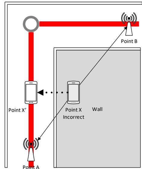
Figure 37 - Cornered hallway with two-point position snapping (*Incorrect and projected X location*)
