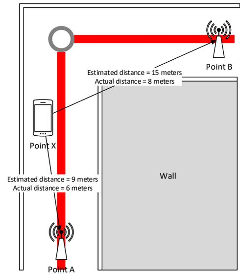
Figure 36 - Cornered hallway with two-point positioning (*Actual Point X location*)
