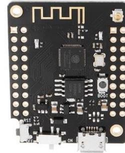
*Figure 11 - Wemos TTGO Mini ESP32 Development board.*
