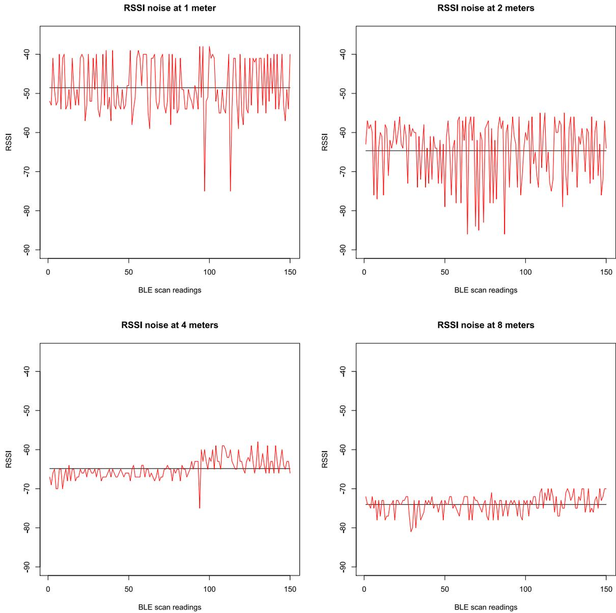
*Figure 17 - RSSI noise measurements over 1, 2, 4- and 8-meter distance*
