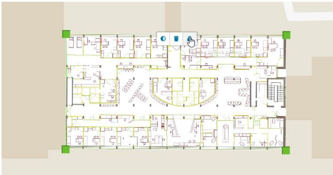
Figure 50 - Aligning a floor plan to the contours on OpenStreetMaps
