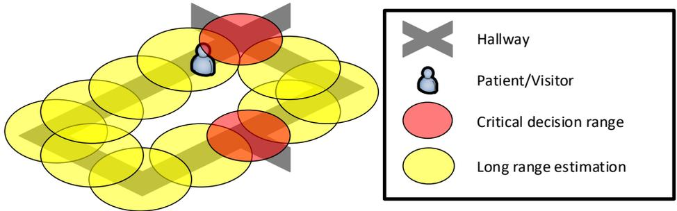
Figure 8 – Cell identification in combination with RSS trilateration inside a hallway
