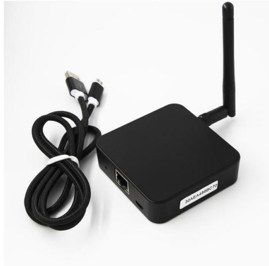
*Figure 2 - Accuware's BLE v3 tracking node with ethernet and Wi-Fi connection (Accuware Inc., 2018)*
