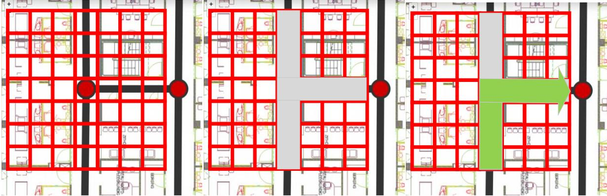
Figure 39 - Mini map creation based on routes. (1) 7x7 pixel grid with a size of 14mx14m, (2) Grid with background context, (3) Grid with directional arrows on top of the background context
