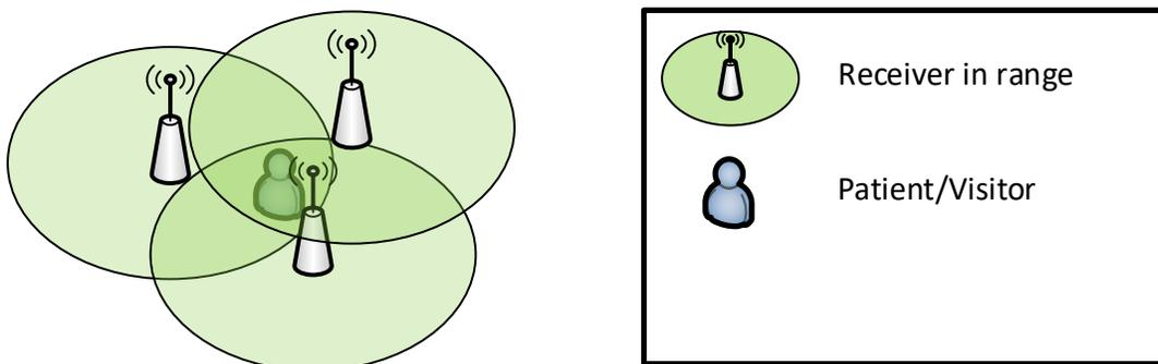
*Figure 6 – Received signal strength positioning*
