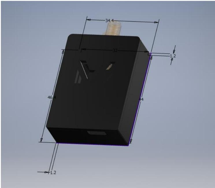
*Figure 47 - Scanner node enclosure assembly*
