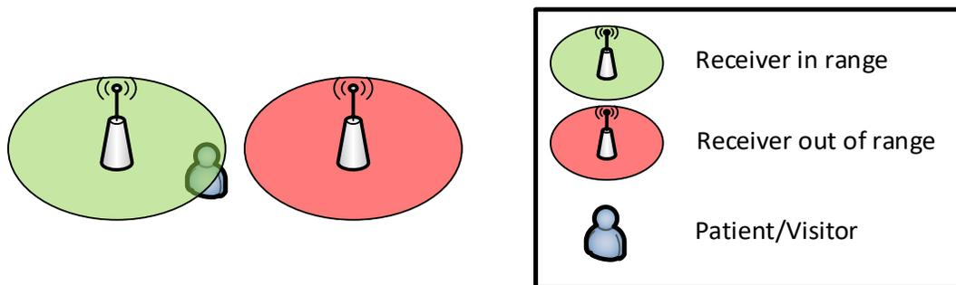
*Figure 3 – Cell identification positioning example*
