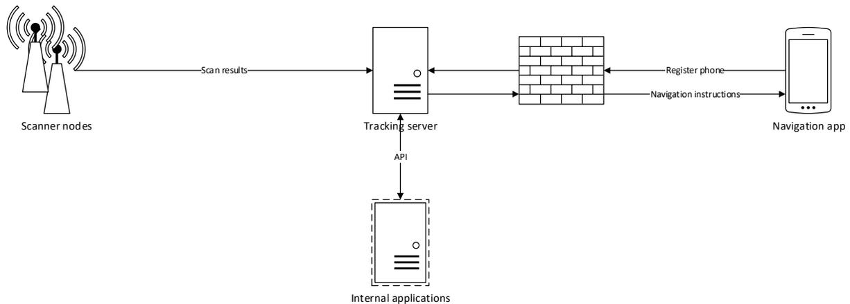
Figure 10 – General system architecture with scanners, tracking server and navigation app
