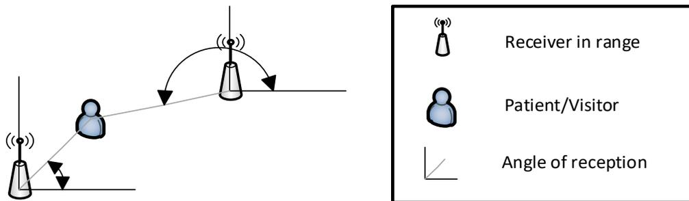
Figure 5 – Angle of arrival positioning example
