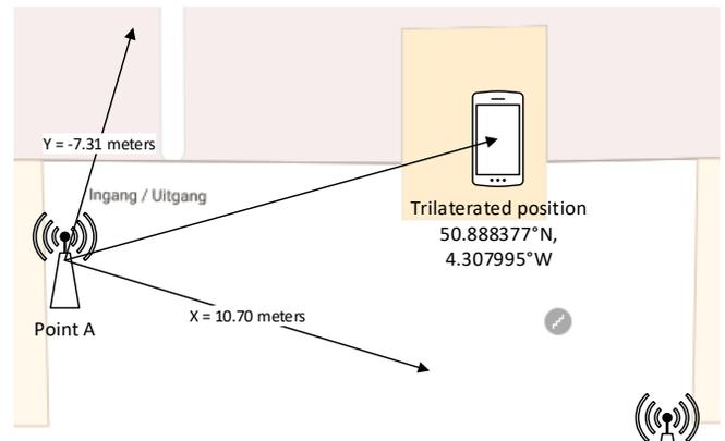
Figure 58 - x, y distance originating from scanner A in the direction of the (x,y) unit vectors
