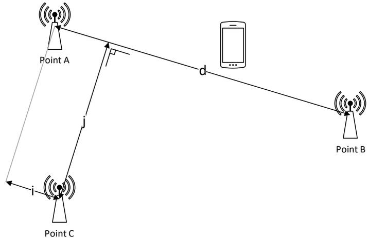
*Figure 57 – Trilateration signed magnitude of the x and y components (i, j)*
