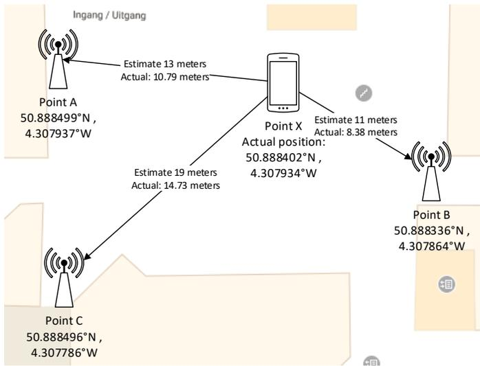
Figure 56 - Trilateration positioning in larger open spaces
