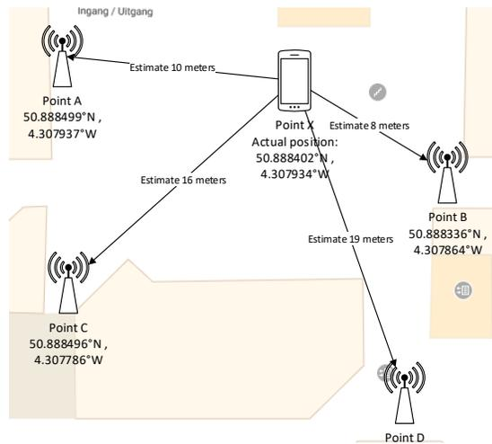
Figure 35 - Selective trilateration with 4 scanners in range
