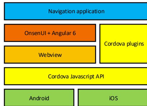
Figure 13 – Smartphone navigation application architecture
