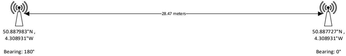
Figure 54 - Two-point calculated distance and bearings
