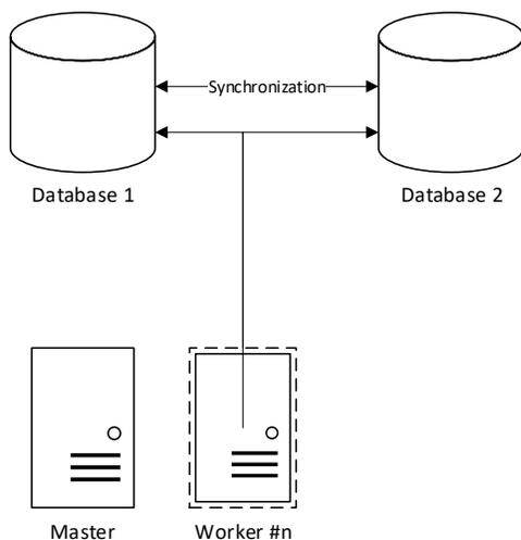
The architecture of the tracking server is shown in Figure 12. Two (MySQL) databases are set-up as a single load balanced database that is accessed by multiple workers. They contain all the persistent data of the system ranging from the latest readings of scanners to login sessions of the configuration.
