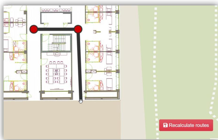
Figure 26 - Route configuration, holding Shift while creating a new edge. Recalculate button is shown
