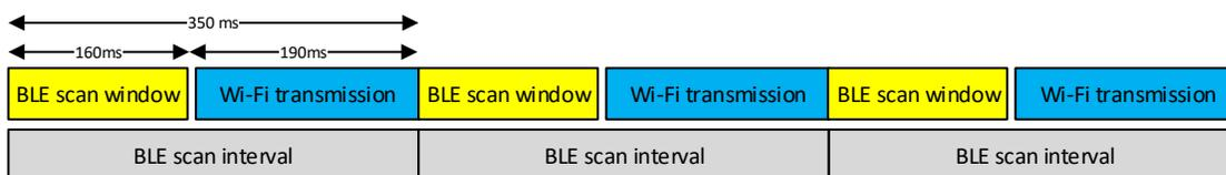
Figure 16 - BLE scan window and interval
