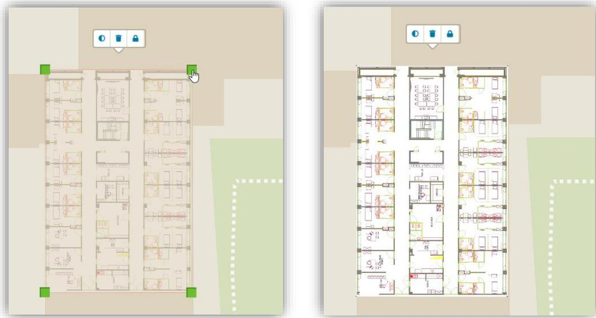
*Figure 24 - Screenshots of georeferencing a network floor plan. Left while it is being positioned and right after locking it*
