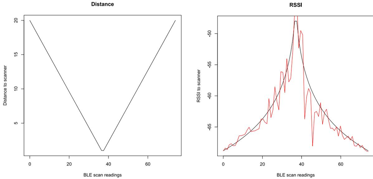
Figure 18 - Simulated Kalman filter experiment. Starting point distance and RSSI (with noise).
