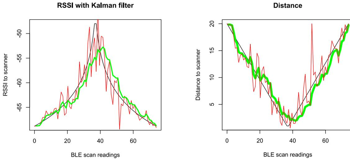
Figure 19 - Filtered RSSI (green) and converted distance using the modified Kalman filter
