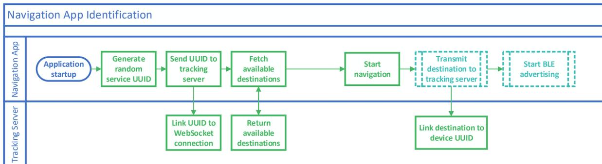
Figure 44 - Navigation app identification process model and communication
