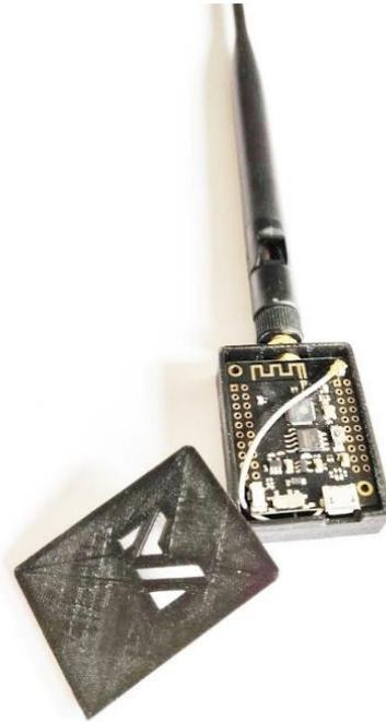
*Figure 14 - Wemos ESP32 development board inside a 3D printed prototype casing*
