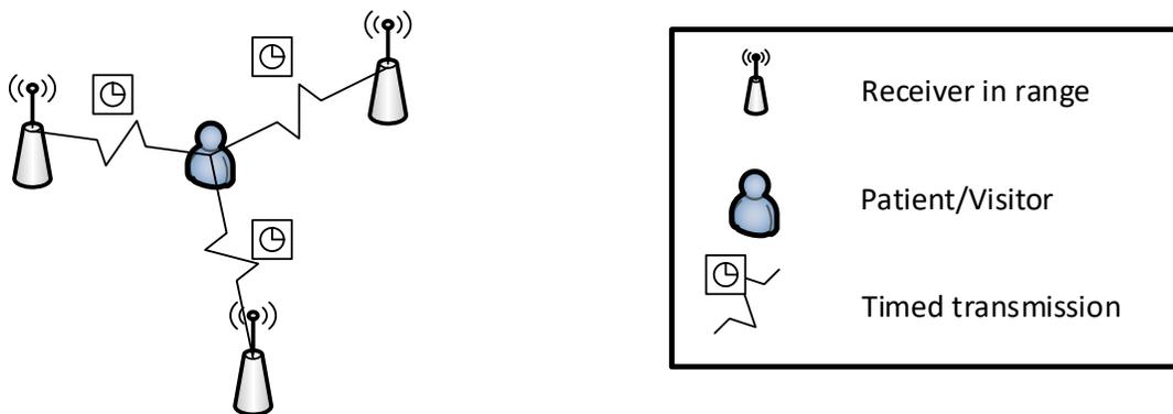
Figure 4 – Time of arrival positioning example
