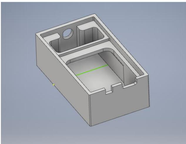
*Figure 48 - Scanner node enclosure with battery (Used for experimentation)*
