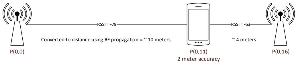
Figure 9 – Position estimation between two stationary receivers in the same X dimension
