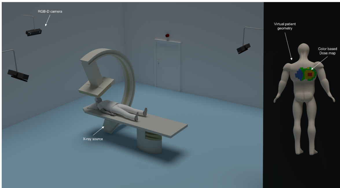
Figure 2 – Schematic representation of the dose calculation system setup in an interventional radiology room with the results displayed on the right side. A short animation video illustrating the setup can be found at https://youtu.be/yG9pJMmbv69
