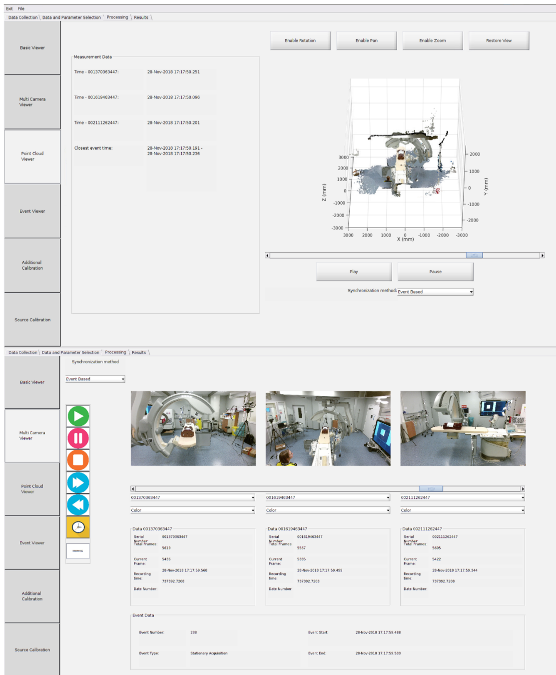
Figure 19 – Two of the viewer modules, the point cloud viewer to inspect registration at the top and multi camera viewer to inspect the synchronization at the bottom, this is an optional feature for the advanced user
