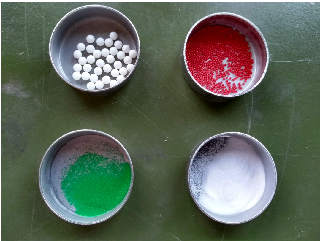
Figure 4.1: The 4 different kinds of MP that are used during the experimental phase of this research: white PP ( 2.45 \pm 0.05 \text{ mm} , top-left), red PE ( 600\text{-}710 \text{ }\mu\text{m} , top-right), green PE ( 90\text{-}106 \text{ }\mu\text{m} , bottom-left) and white PE ( 10\text{-}45 \text{ }\mu\text{m} , bottom-right) (Cospheric, USA).
