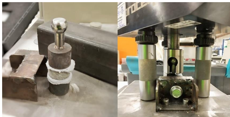
Figure 26: Interlayer tensile strength test setup
