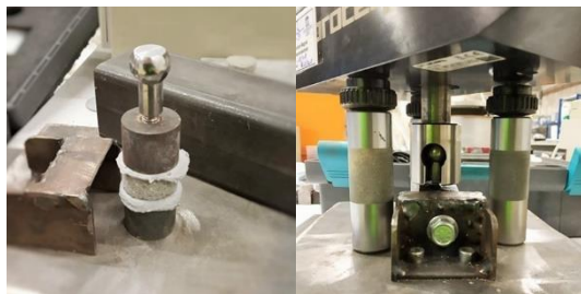
Figure 6: Interlayer tensile strength test setup
