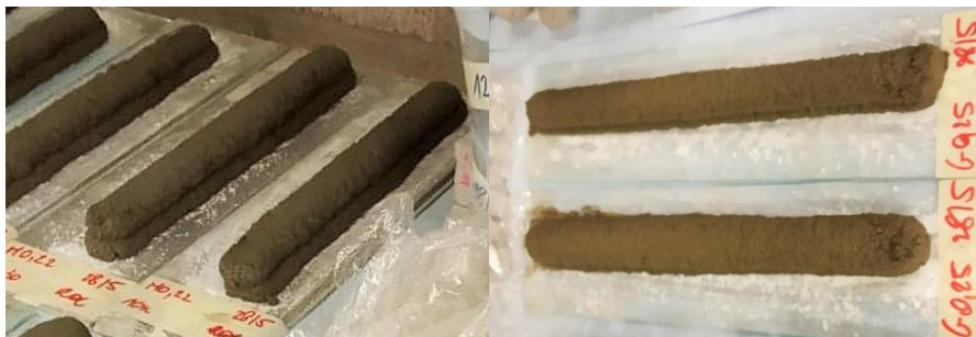
Figure 34: Visual inspection of the stability of the first layer when a second one is superposed
