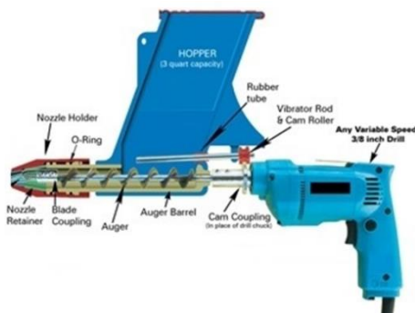
Figure 2: Quikpoint mortar gun [50]
