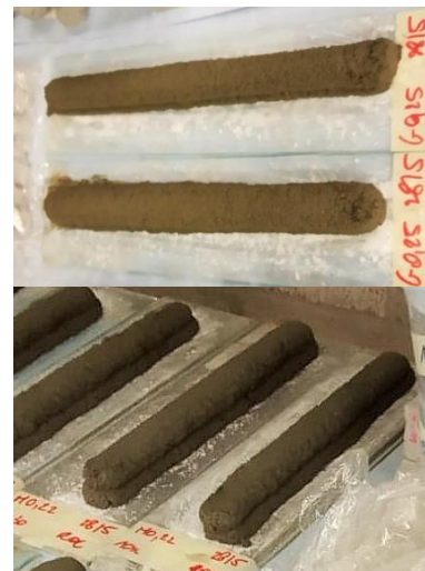
Figure 9: Visual inspection of the stability of the first layer when a second one is superposed (above: G025; below: M022)
