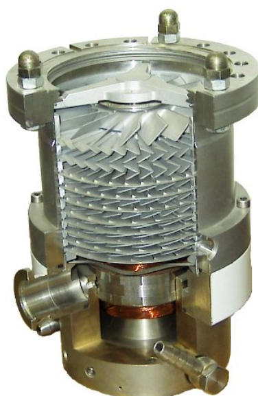
Figure 4.1: Interior view of a turbomolecular pump. Different rotor sizes can be seen.
