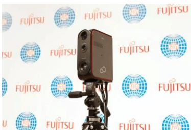
Picture 1 – Fujitsu's 3D sensing device, consisting of a camera, a Lidar pulse transmitter and a receiver (Sarazen, 2019).
