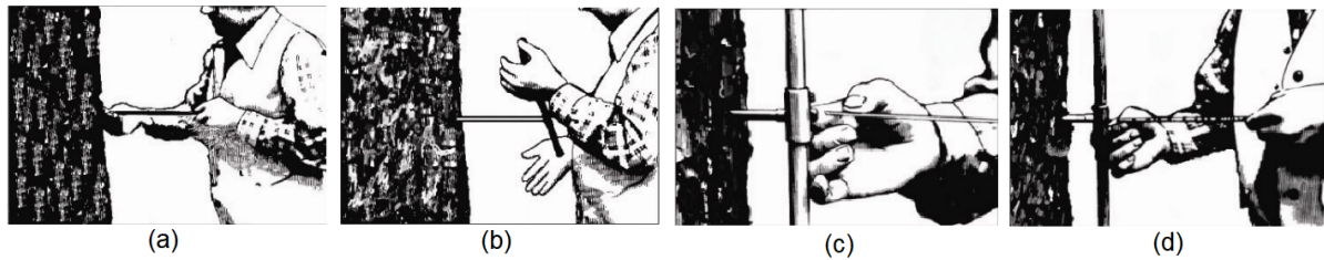
Figure 3.4: Instructions for collecting wood samples. (a) Place the tip of the borer in an angle of 90^\circ at the appropriate boring height. Grasp the shaft of the auger with one hand and hold the handle center with the other. (b) Apply inward pressure to help the auger tip penetrate the outer bark. Keep applying this pressure while rotating the increment borer until the threads engage and the auger tip enters the tree. (c) Slide the extractor into the auger and turn the handles counter-clockwise for two turns. (d) Pull the extractor cap gently until the core breaks free (Grissino-Mayer, 2003). Figure adopted from Chave (2005).
