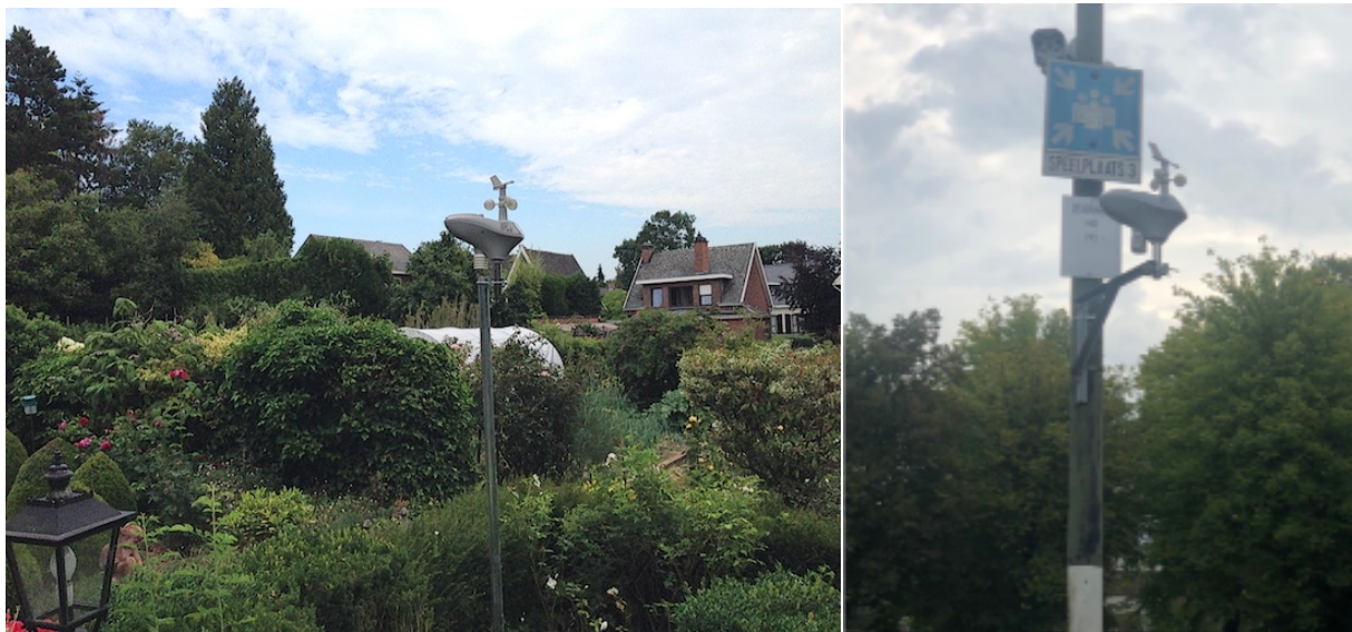
Figure 3.5: Example of installed weather stations in a private garden (left) and a semi-public playground (right).
