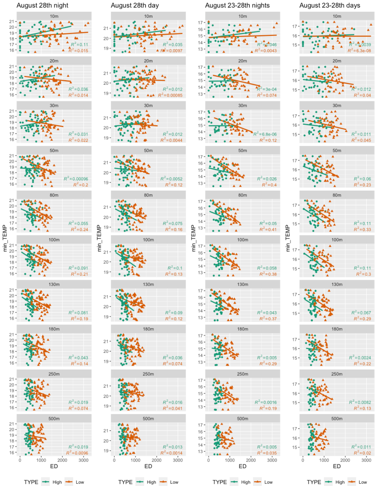
Figure 8.7: Scatterplots between minimum temperature and the edge density of high and low green for multiple spatial (10m, 20m, 30m, 50m, 80m, 100, 130m, 180m, 250m and 500m) and temporal scales (August 28 th night/day and August 23-28 th nights/days).
