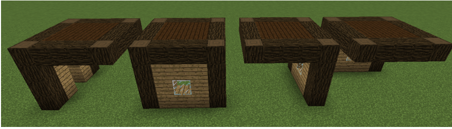
Figure 4.1: Rules for the rightmost ceiling shape in the shape set 3.6a from example 3.1a. There is a rule for every other shape in the shape set that makes contact with this shape. The rule produces the new shape in the same position and orientation relative to their positions in the example structure.
