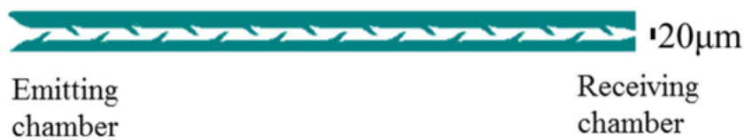
FIGURE 2.14: Barbed channels trapping neurites in one direction but letting them pass in the other. Reprinted by permission from Frontiers in Neuroscience [43].
