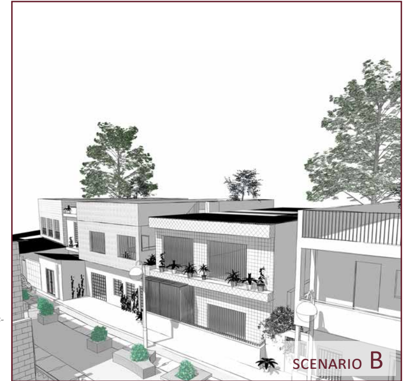
► Image 145 Axonometric view the transformation with a balcony garden, the two middle buildings do not share a wall
