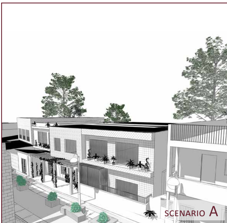
► Image 144 Axonometric view of side garden system, the two middle buildings share a wall
