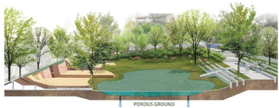
Schematic section of a floodable plain - Chulalongkorn University Centenary Park © G49 Co., Ltd.
