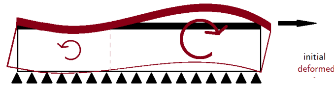
Figure 23: Illustration of the force distribution in the pad that exhibits interfacial cavitation as a failure initiation mode. The pulling of the pad parallel to the substrate combined with the boundary conditions at the adhesive surface creates internal stress distributions with resulting couples in the pad. This results in the formation of the interfacial cavitation.
