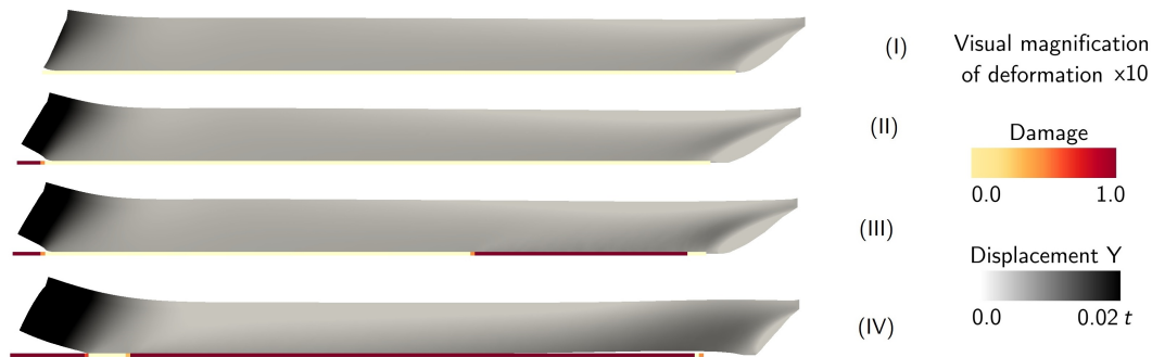
Figure 33: Failure sequence of the simulation with parameter values (\beta, \alpha, L/t, \theta, \zeta, \gamma, \kappa) = (20, 2, 15, 0.5 \times 10^{-3}, 60 \times 10^{-3}, 4.8, 0.4) that exhibits curling with interfacial cavitation. The imposed displacement is varied from Figure (I) to Figure (IV). At every stage, the (magnified) deformation of the pad is shown, with additional shading for the vertical displacements. On the bottom of the pad, the level of damage of the cohesive zone is shown. In Figure (I) the pad is placed under loading and no damage is observed yet, a vertical lift at the surface near the opposite end is observed. (II) The first small detachment region near the opposite end starts developing. (III) Sudden propagation of failure of the interfacial cavitation mode near the pulling. (IV) Interfacial cavitation detachment and curling detachment merge. The pad is fully detached.
