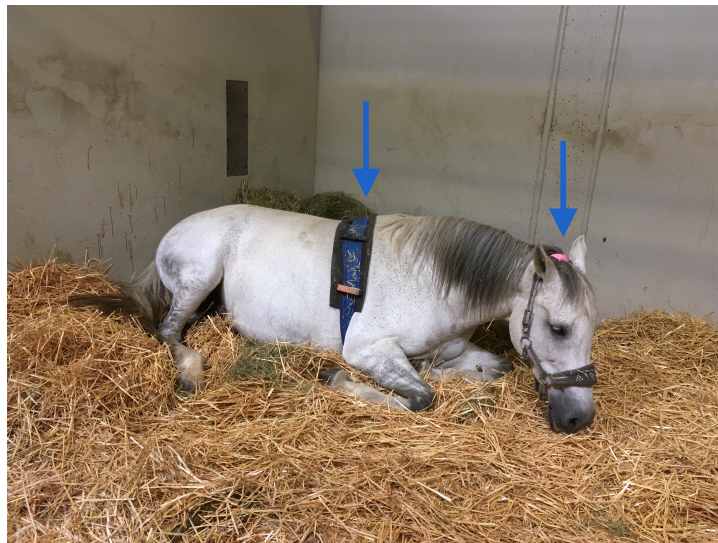
Figure 2.3: Placement of the accelerometers
