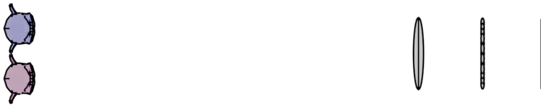
(b) Top view of the setup. From left to right: subject, main lens, micro-lenses and image sensor.
