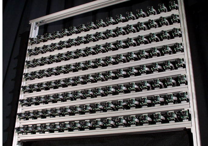
(a) The Stanford Camera Array. The baseline between the cameras can be changed.
