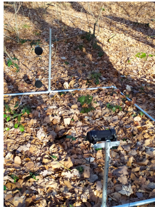
Figure 3.7: Picture of the measurement set-up as it is used, this set-up example has the Nordtest-method standardized dimensions. From left to right: the metal frame, microphones, and source.
