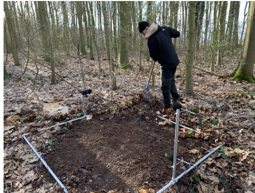
Figure 3.10: Example of manually removing the litter layer of a sample plot of northern red oak, Quercus rubra , to measure the acoustic properties of the bare forest soil.
