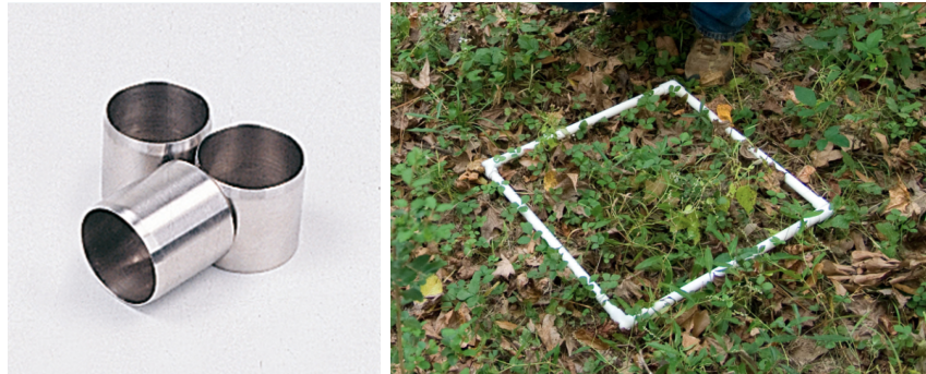
Figure 3.9: Kopecky rings used for gathering soil for the calculation of the moisture content, are typically 100 \text{ cm}^3 (left) [94] A sampling square that is used to make sure every time the same amount of litter is observed and collected. The one used is 20 \times 20 \text{ cm} (right) [95].
