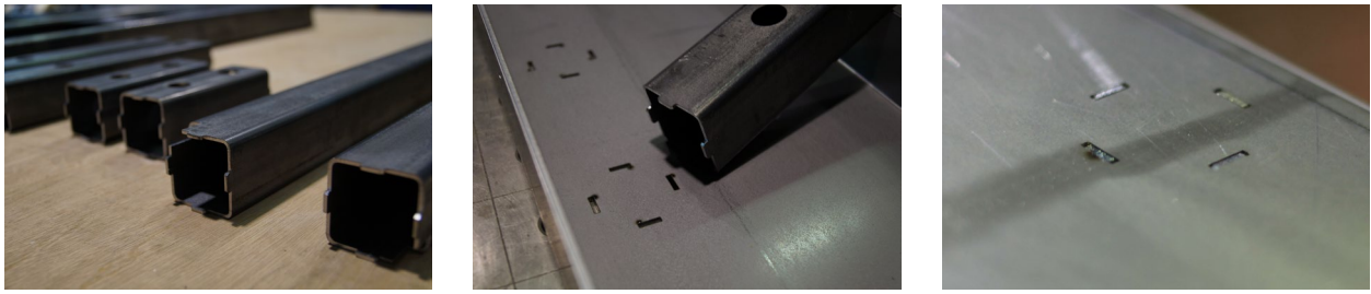
Figure 29: Tab and slot assembly.
