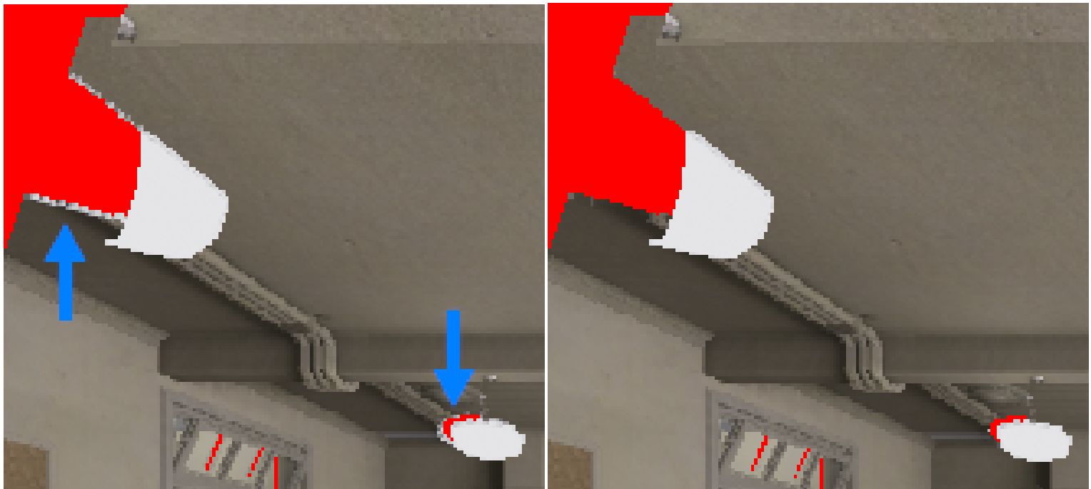
Figure 6.6: DIBR result when using one input image, on the left without the preprocessing step from Section 4.4 and on the right with. The red areas behind the lamps were occluded from the perspective of the input camera, but are visible for the virtual camera. The white edge artefacts on the left image (indicated by blue arrows) are caused by a difference between the depth map and the input image. To be precise, these white artefact pixels are white on the input image because they belong to the lamps, but the depth map gave them a depth value of the ceiling behind the lamp, resulting in these pixels being placed on the ceiling in the virtual image rather than on the lamp.
